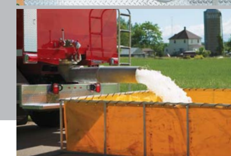
Pierce's exclusive rear 10" tank dump with manual valve and 90-degree directional elbow.
