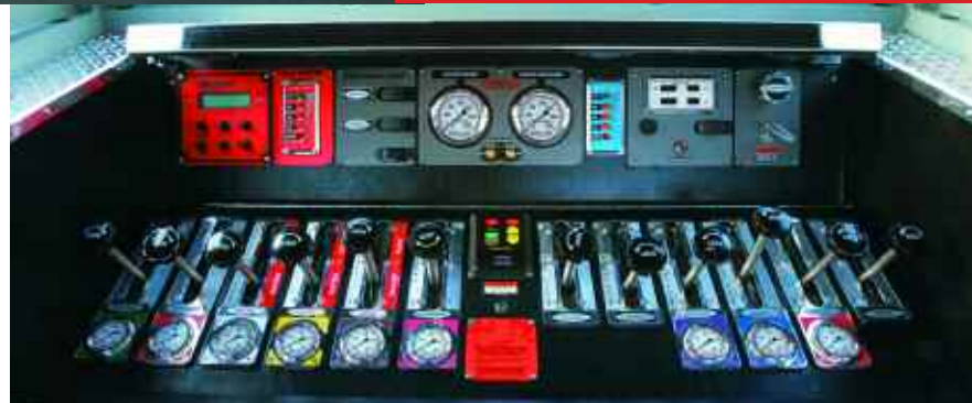
Top mount control panel with a color-coded, organized panel and sealed levers.
